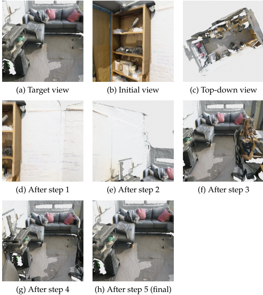
Figure 8 | IVP example. Our trained Qwen2.5-VL-7B plans view changes from (b) to match (a) in 6 turns. Final viewpoint error: 0.061 m / 0°. Success.
